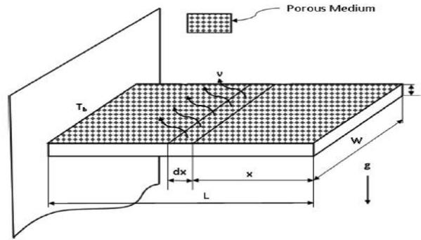
Figure 1: Schematic of the longitudinal natural convection porous fin
