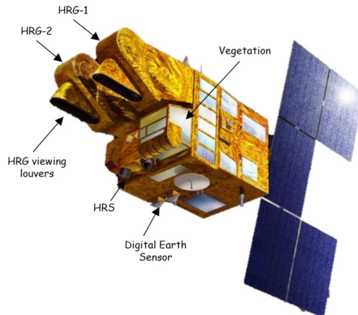
**Figure 1: Instruments on-board SPOT 5 satellite (Modified after Satellite Imaging Corporation, 2015)**
