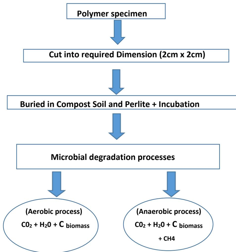
Figure 1: Biodegradation process of polymer or plastic material
