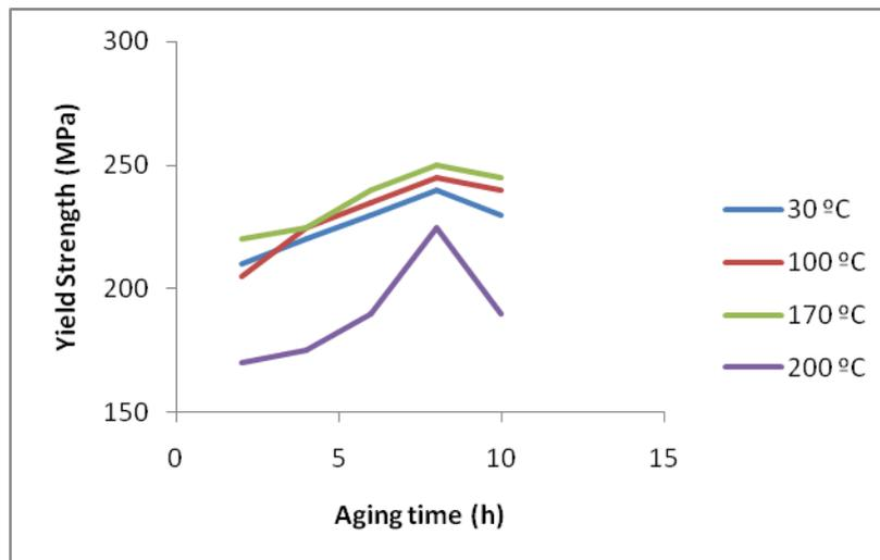
Figure 3: Effect of aging temperature on the yield strength of LM12
