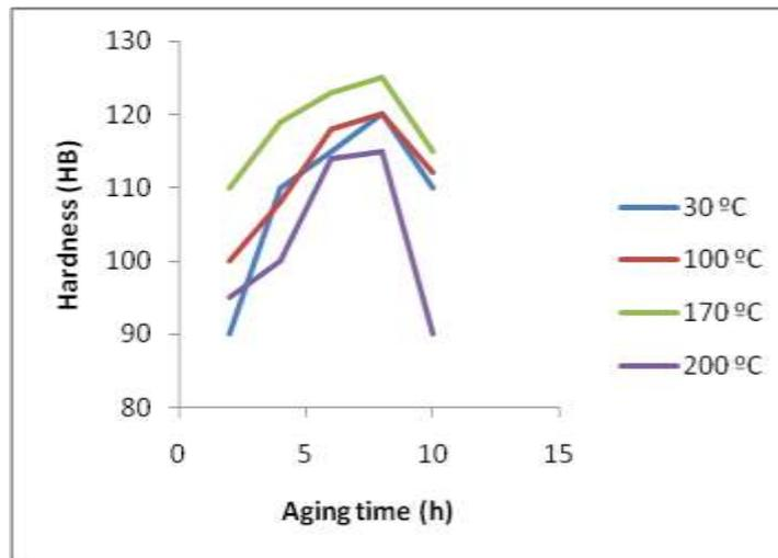
Figure 2: Effect of aging temperature on the Hardness of LM12
