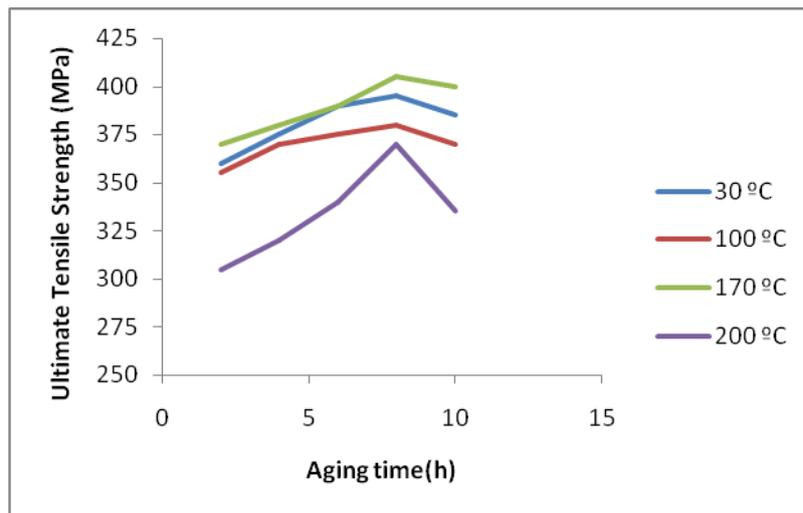
Figure 1: Effect of aging temperature on the UTS of LM12
