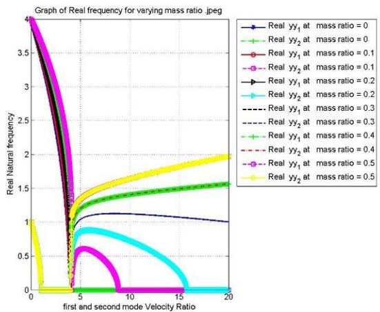
Figure 7(a): Effect of mass ratio on real frequency for Modified Tai-Ping Chang model
