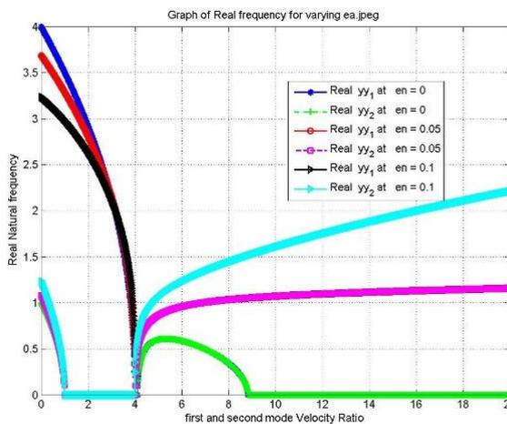
Figure 2(a): Effect of non-local parameter on real frequency for Modified Haw-Long Lee model
