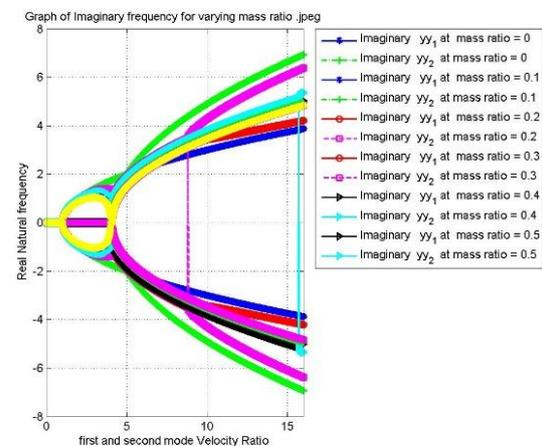
Figure 8(b) Effect of mass ratio on imaginary frequency for Modified Haw-Long Lee model
