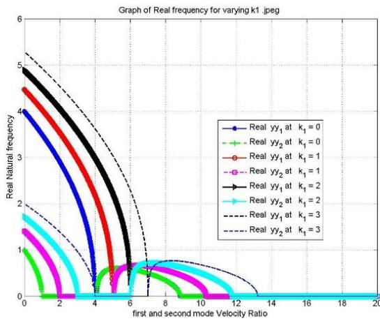
Figure 4(a): Effect of Pasternak constant on real frequency for Modified Haw-Long Lee model
