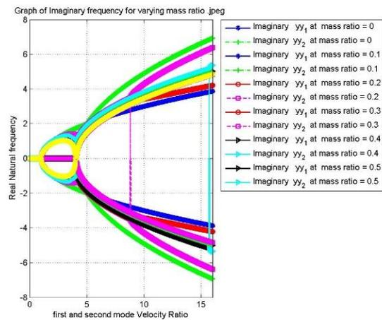
Figure 7(b): Effect of mass ratio on imaginary frequency for modified Tai-Ping Chang model
