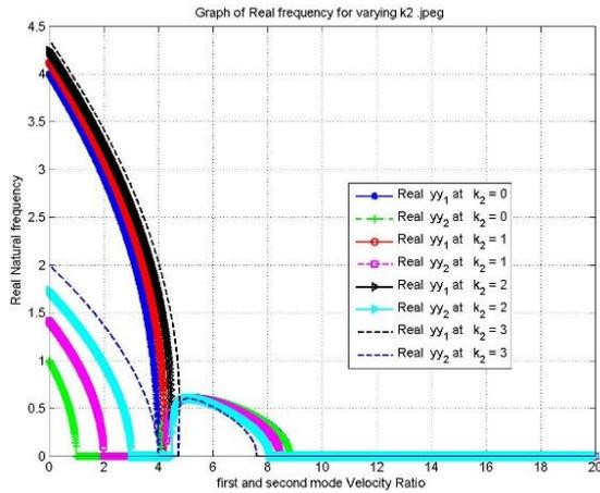
Figure 6(a): Effect of Winkler constant on real frequency for Modified Haw-Long Lee *et al.* model
