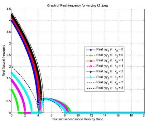
Figure 5(a): Effect of Winkler constant on real frequency for Modified Tai-Ping Chang model
