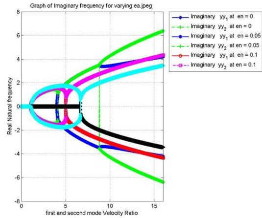
Figure 1(b): Effect of non-local parameter on imaginary frequency for Modified Tai-Ping Chang model
