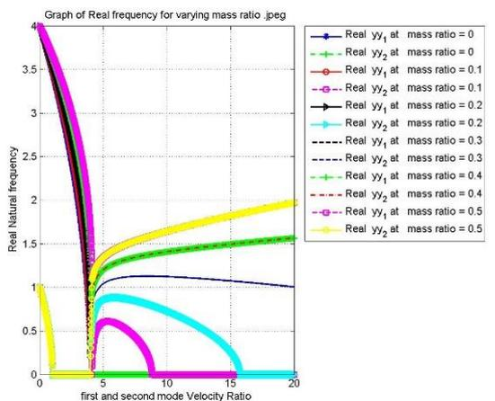
Figure 8(a): Effect of mass ratio on real frequency for Modified Haw-Long Lee model
