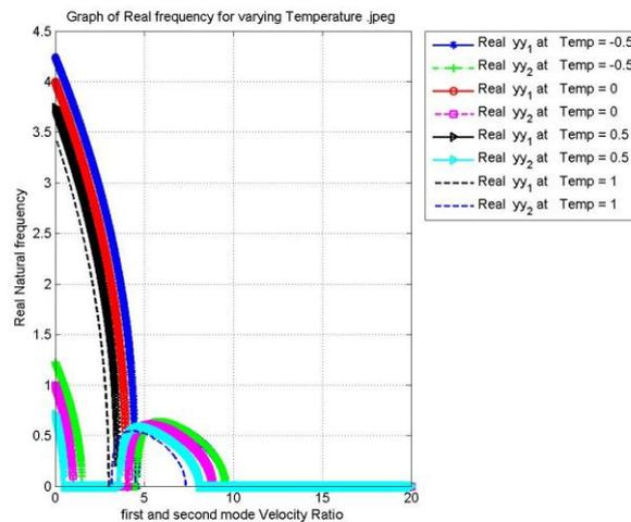
Figure 10(a): Effect of temperature on real frequency for Modified Haw-Long Lee et al model
