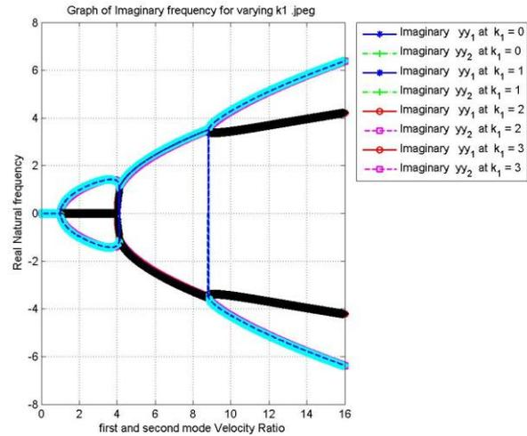
Figure 3(b): Effect of Pasternak constant on imaginary frequency for modified Tai-Ping Chang model
