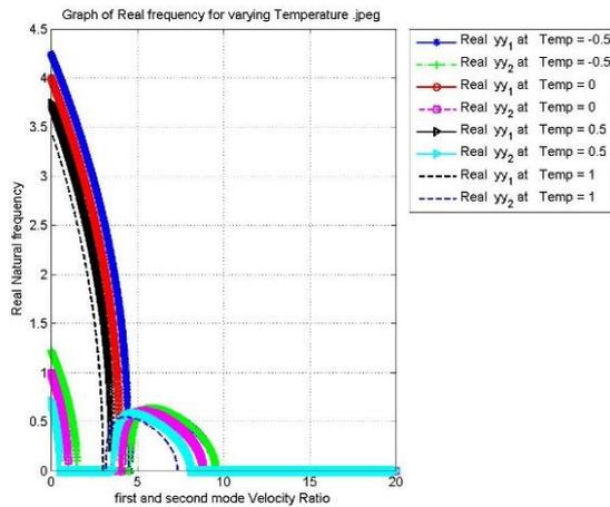
Figure 9(a): Effect of temperature on real frequency for Modified Tai-Ping Chang model
