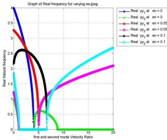
Figure 1(a): Effect of non-local parameter on real frequency for Modified Tai-Ping Chang model
