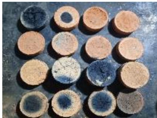
Figure 11: Result of firing at the rate of 150 °C per hour before oven drying
