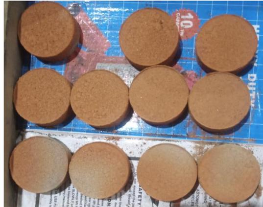
Figure 12: Filters produced from oven drying at 50 °C before firing at the rate of 75 °C/hr
