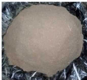
Figure 2(b): Pulverized coconut shell
