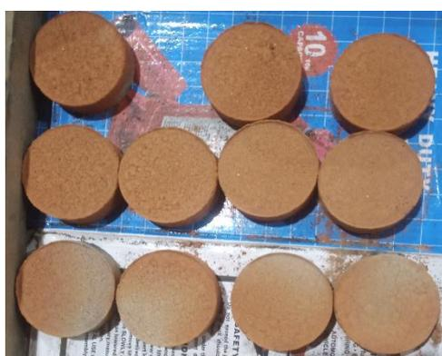
Figure 5: Fired filter samples
