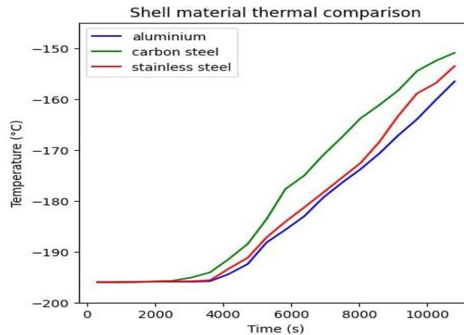
Figure 5: Cryogenic Temperature Change with Time for different Cryotank Materials
