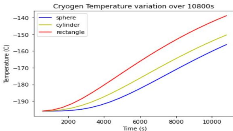
Figure 3: Cryogenic Fluid Temperature Variation with Time
