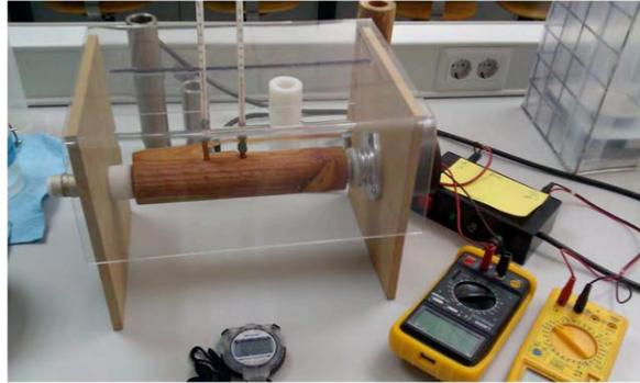
Figure 2: Experimental Determination of the Thermal Conductivity of a Cylindrical Polyethylene Material (Ortuno *et al.*, 2011)
