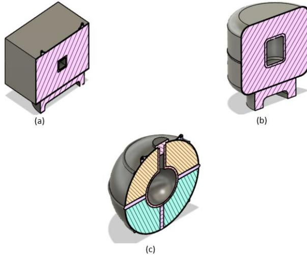
Figure 1: Physical Model of Different Shapes of Cryotanks (a) Rectangular (b) Cylindrical (c) Spherical
