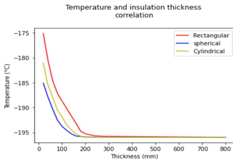
Figure 4: Effect of Insulation Thickness on Cryogenic Temperature
