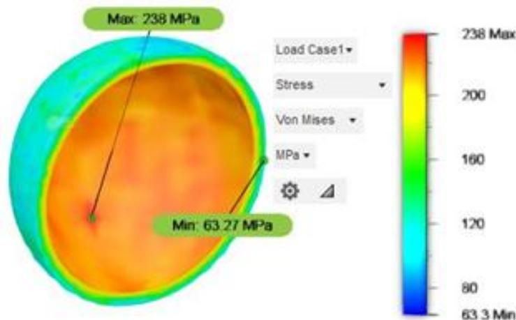
Figure 6: Thermal Stress Distribution (Aluminium Inner Shell)
