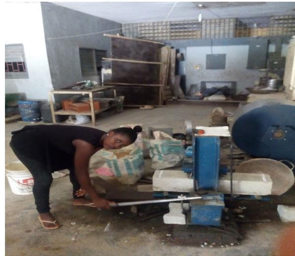
Plate 4: Flexural strength test in process
