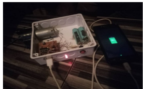
Figure 9. The photographic view of the fully charged proposed device with mobile phone connected and being charge
