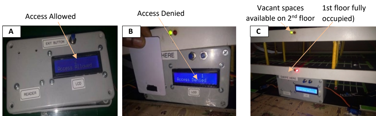
Figure 1: Different displays at the entrance of car park (A) Valid RFID card, (B) Invalid RFID card, (C) Space availability
