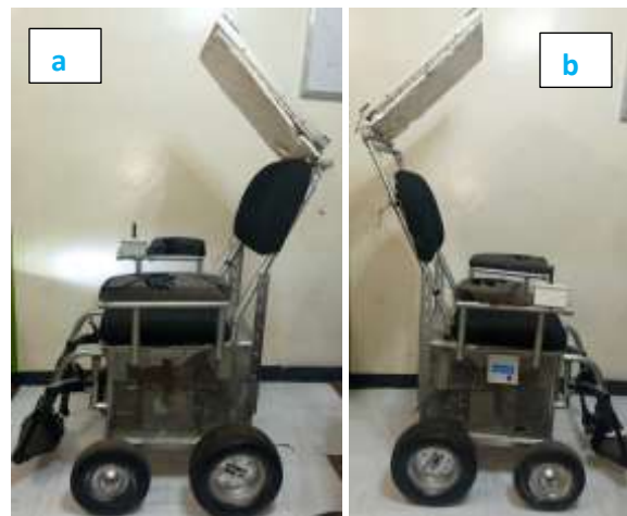
Figure 6: (a) Left View of the Finished EDW (b) Right View of the Finished EDW with solar PVC roof
