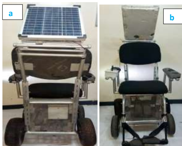
Figure 7: Rear View (a) and Front View (b) of the Finished EDW with solar PVC roof
