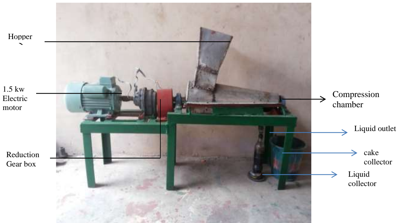
Figure 3: Fabricated Cashew Nut Shell Liquid Expeller
