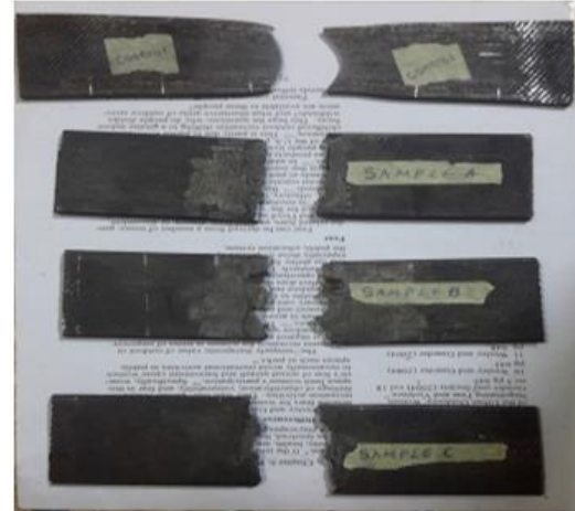
Figure 2: Tensile Test Fractured Samples
