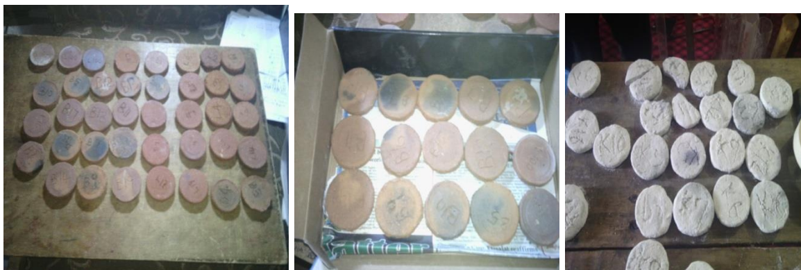
Plate 1: Disk-shape filters with different material compositions
