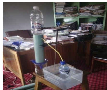
(b) Filtration system with PVC as storage device
