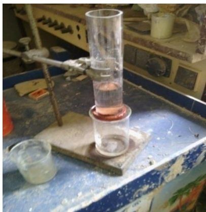
(a) Filtration system with glass as storage device
