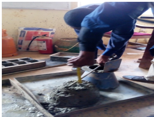
Figure 5: Slump test on fresh concrete
