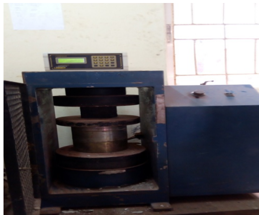
Figure 6: Compressive strength test on cured concrete
