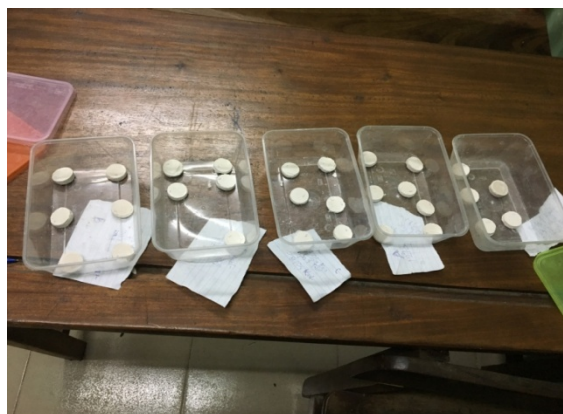
Figure 1: Picture showing the samples after the pressing in a uniaxial press
