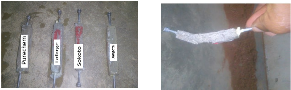
Figure 9: Appearance of cement paste prism exposed to sulphate attack (a) Other sulphate attack (b) MgSO_4 attack
