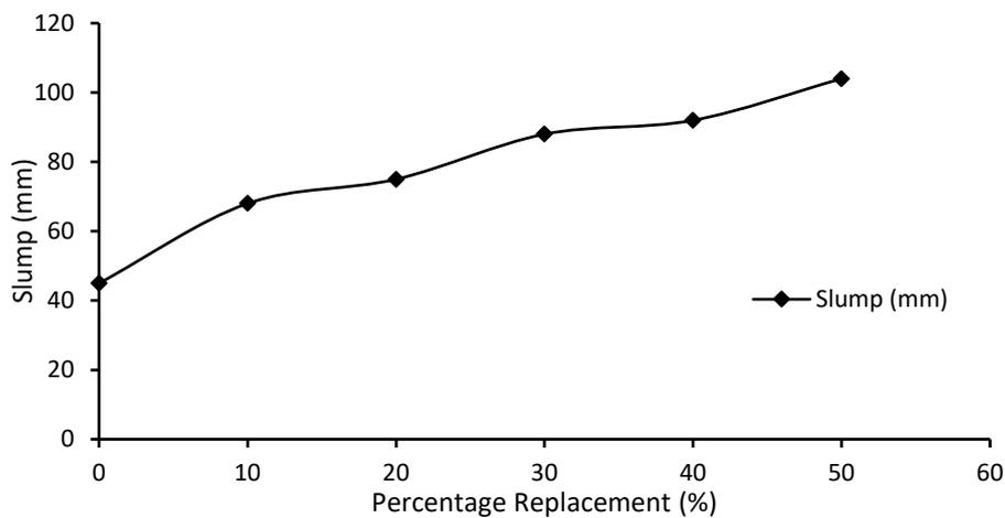
Figure 2: Variation of slump values at different POFA percentage replacement
