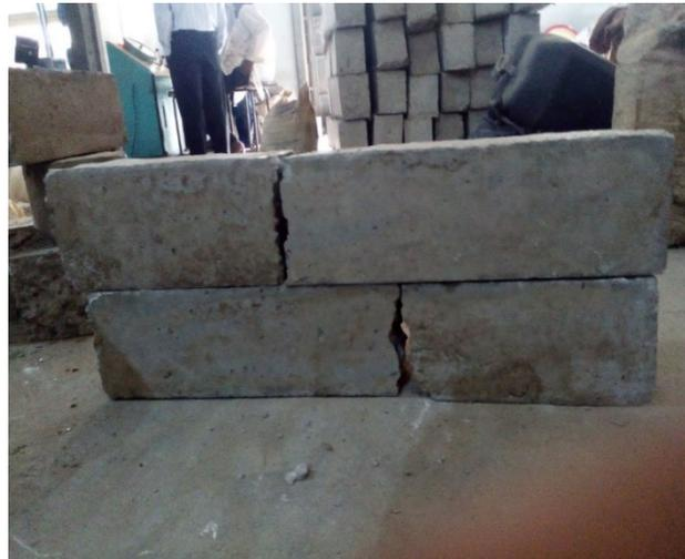
Plate 5. Failure pattern of the beams
