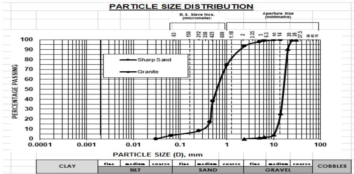
Figure 1: Aggregates Particle Size Distribution Curve
