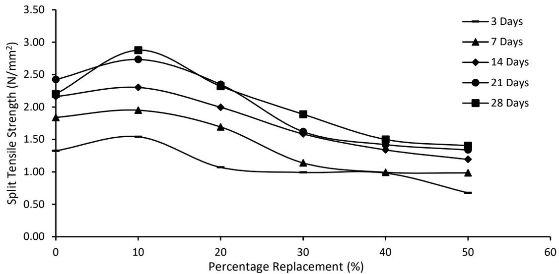
Figure 4: Variations of Tensile Strength at different Cement Fineness Zone
