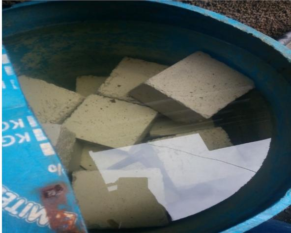
Plate 1: Curing of concrete cubes
