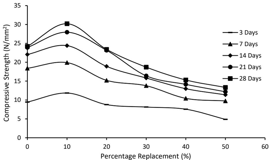
Figure 3: Variations of Compressive Strength at different Cement Fineness Zone
