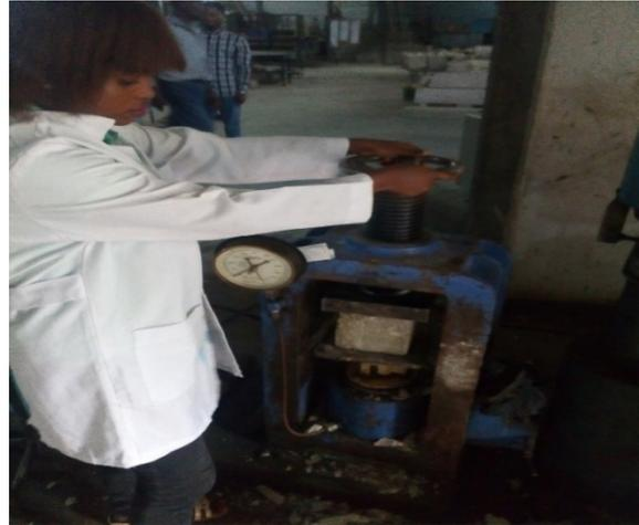
Plate 2: Crushing of Cubes
